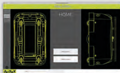
From the Map Editor it is possible to define and edit the predetermined paths of the robots, the docking points and the navigation rules in each area of the work area
